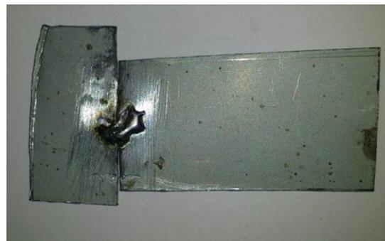
Gambar 4.5 Hasil pengelasan soldering 6 Ampere
